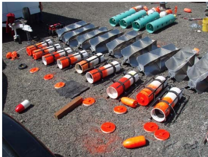
Figure 3. Drogues with aluminum and PVC drag elements. Vertical dimensions of both types were identical.
